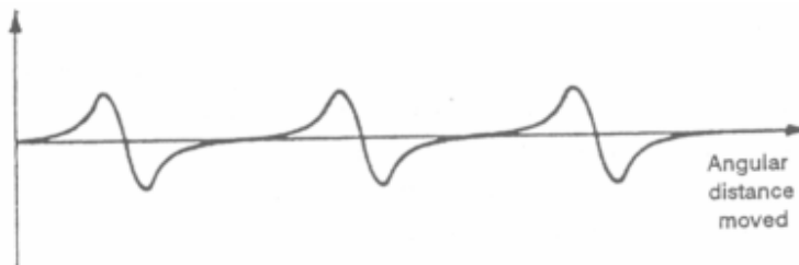
Figure 14-8. Pattern of Flux Change With Rotation of a Variable-Reluctance Transducer.
